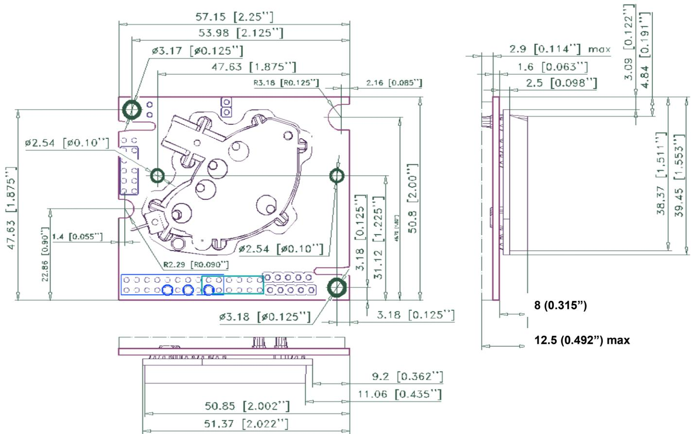
Figure 4. CO<sub>2</sub> Engine<sup>®</sup> K30 mechanical drawing.
